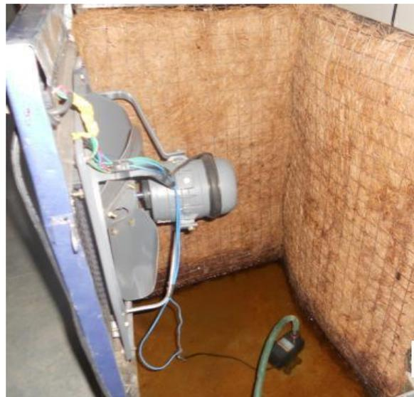
**Fig. 5 Test rig of Evaporative cooler**
