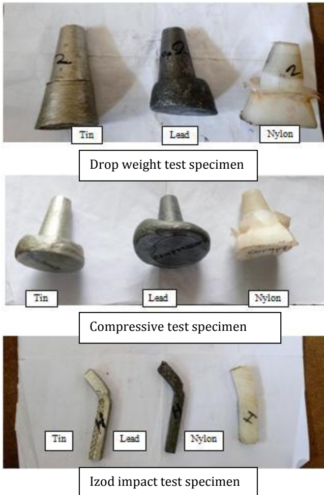
Fig.6. The deformed shapes of tested specimens
