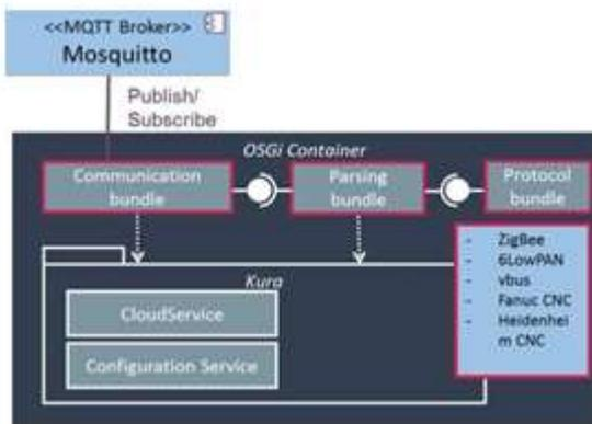
Figure 4: The structure of a communication agent
