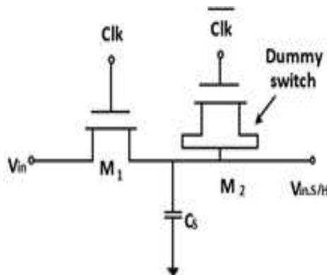
Fig. -2: Schematic of Sample and Hold circuit
