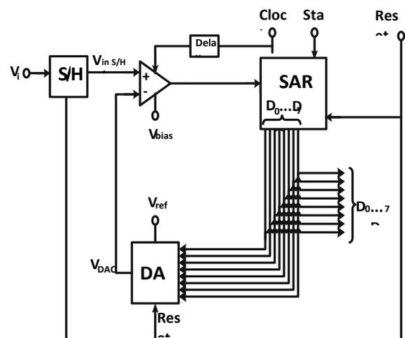
Fig. -1: Schematic of the proposed 8-bit SAR ADC
