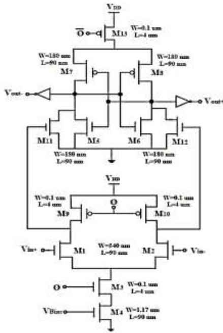
Fig. -4: Schematic of Double Tail Dynamic Latch Comparator
