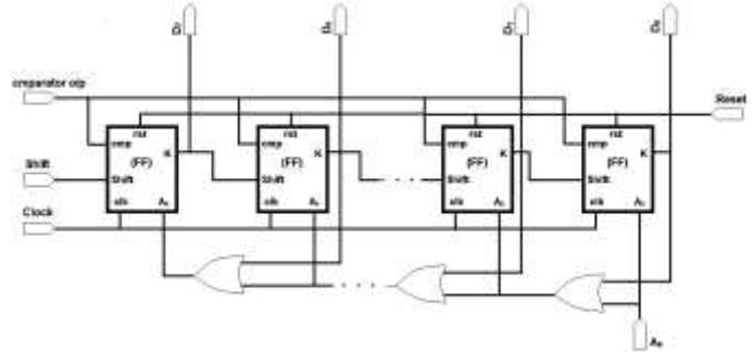
Fig. -6: Schematic of SAR control logic
