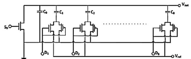
Fig. -8: Schematic of binary weighted switched capacitor array DAC
