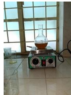
Fig 5.2.1: Oil sample being heated
