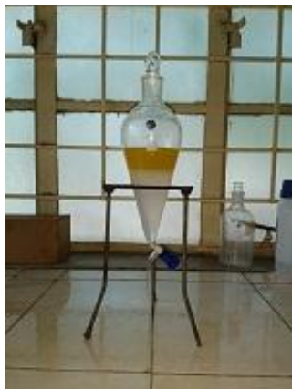
Fig. 5.2.3: Separation of biodiesel and water after final wash
