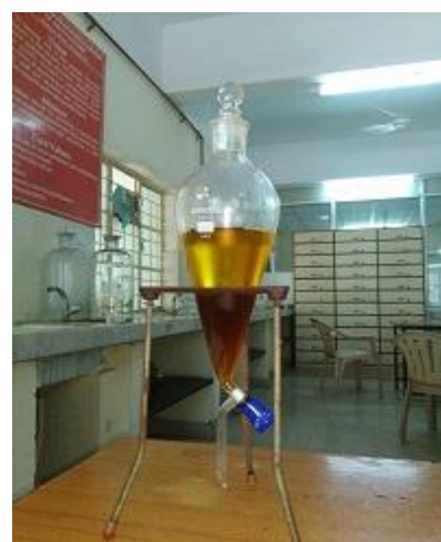
Fig5.2.2 Biodiesel and glycerol separation
