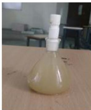
Fig: 1 Density Bottle fill with water
