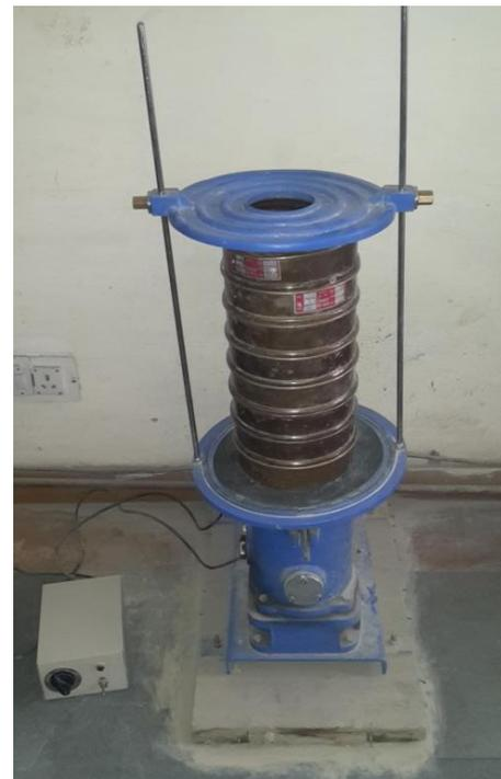
A sieve analysis is a procedure used to assess the particle size distribution of a granular material. The size distribution is often of critical importance to the way the material performs in use
