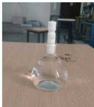
Fig: 2 Density Bottle fill with water and sand
