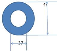
**Fig 1: Evacuated Tube Dimensions 1**
