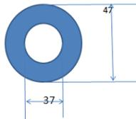
**Fig 1: Evacuated Tube Dimensions 1**
