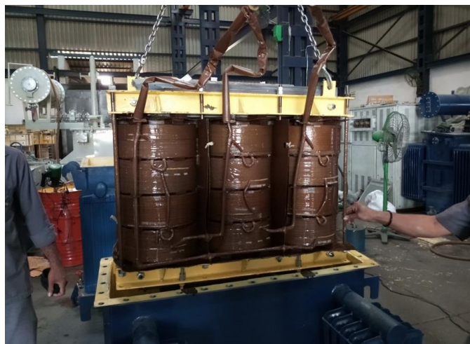
Fig -1: Transformer with mild steel clamping
