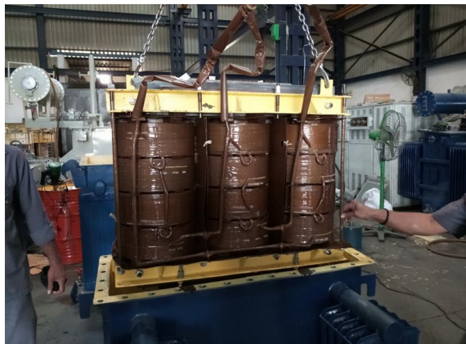
Fig -1: Transformer with mild steel clamping
