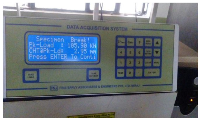
Data acquisition on UTM for deep beam
