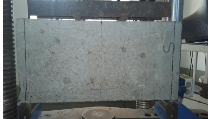
Applying a load on deep beam
