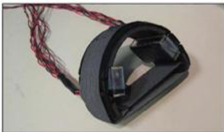
Fig -2: A bio-acoustic sensing array in an armband. (Inside View)[5]
