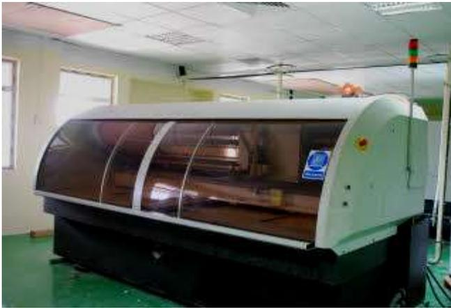
**Fig No. 2 :** Lenz PCB drilling machine
