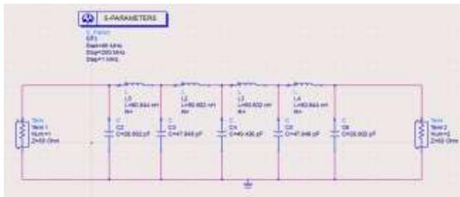
Fig-5: Schematic Design
