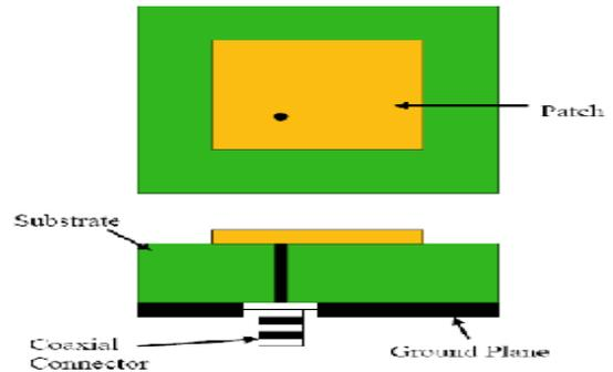
Figure 2.2 Coaxial feed of the antenna
