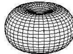
**Figure 1.1** 3D Radiation pattern of a half-wave dipole antenna
