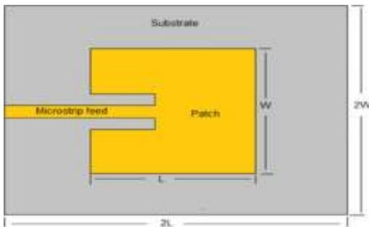
Figure 2.1 Rectangular patch micro strip antenna
