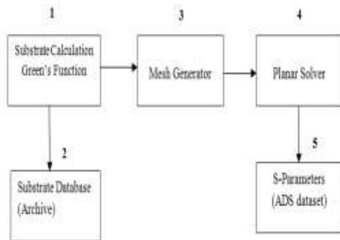
Fig. 3.1 shows the steps of ADS Momentum simulation and outputs
