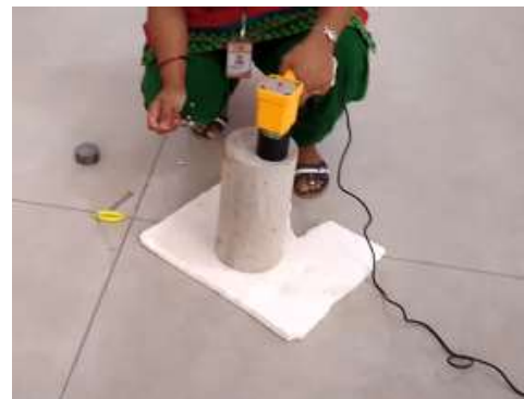
Fig-2: Impact-echo testing on the cylinder
