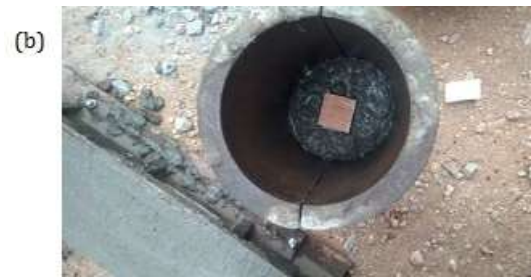
Fig-1: (a) Placing of Styrofoam sheet in the concrete cube; (b) Placing of plywood in the concrete cylinder.
