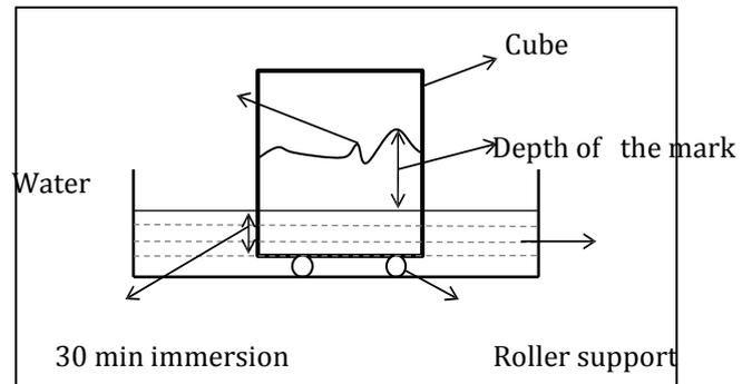
Sorptivity test on cube specimen
