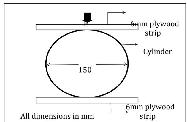
Split tensile test on cylinder specimen
