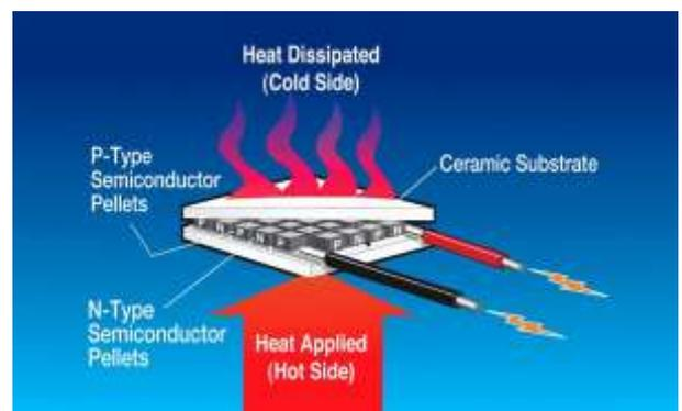
**Fig -1:** Schematic of Thermo Electric Module Operation – Cooling Mode [7]
