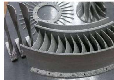
(Fig-2: Turbine Blades made of inconel 600)
