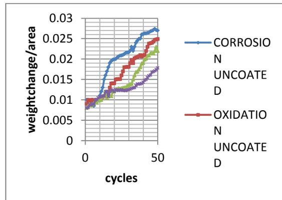
**Chart-1:** Weight change/Area vs. number of cycles plot for coated and uncoated Inconel-600 subjected to cyclic oxidation and corrosion for 50 cycles in air and molten salt environment at  $800^\circ\text{C}$
