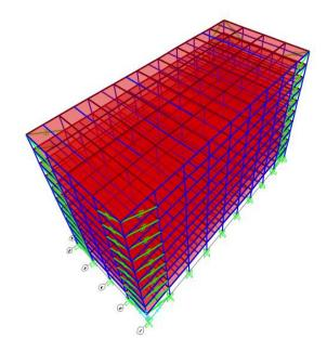
Fig-6. Model of rectangular building with square columns with dampers
