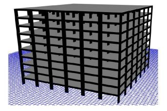
Fig-3. model of square building with rectangular columns without dampers
