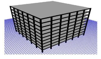
Fig-1. Model of square building with square columns without dampers
