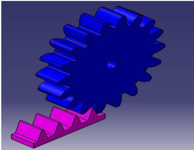
Fig -2: Rack and Pinion
