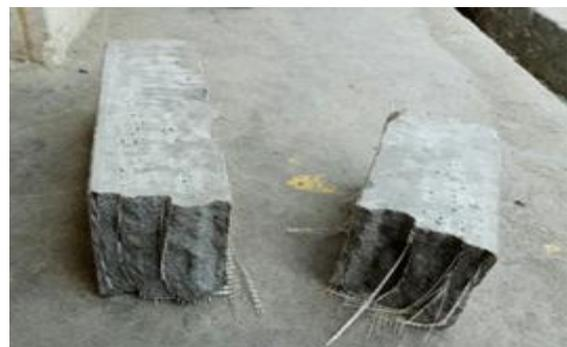
**Fig.4-TRC Beam after Failure**
