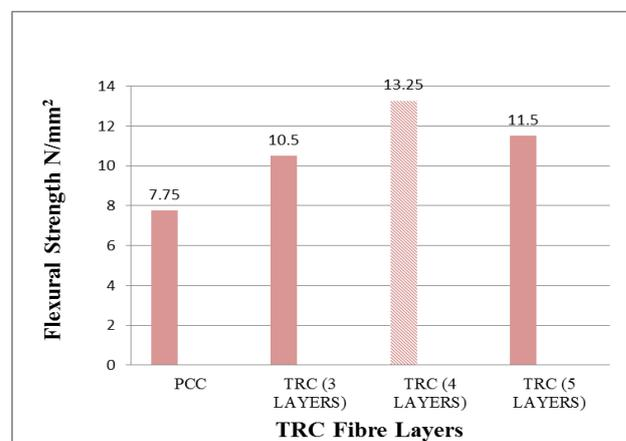
**Fig.5- Flexural Strength of Beam**
