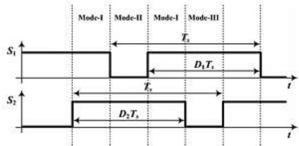
Fig -4: Switching signals for the input boost stage for the proposed converter
