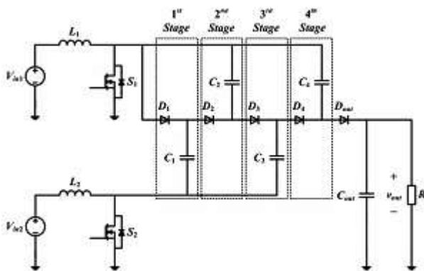
Fig -3: Proposed high-voltage-gain dc-dc converter with four VM stages
