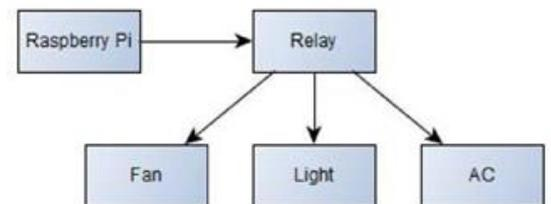
Fig. 2. Block Diagram of Raspberry Pi Connection
