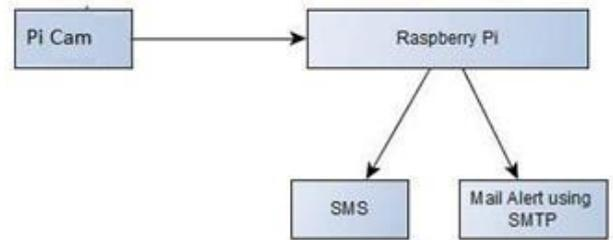
Fig. 3. Block Diagram for intruder alert.
