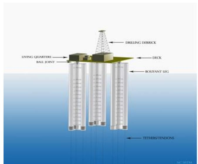
Fig 1: Conceptual view of a Stiffened Triceratops
