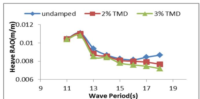
**Fig-7:** Comparison of heave RAO for the BLS unit with and without damper,  $H=19.2\text{m}$
