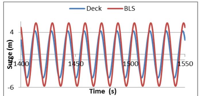
**Fig-4:** Surge response of triceratops without TMD ( $H_{max}=19.2\text{m}$ ,  $T=15\text{s}$ )
