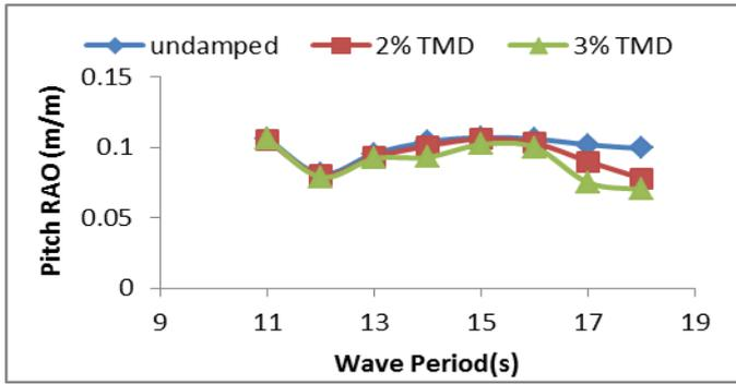
Fig-8: Comparison of pitch RAO for the BLS unit with and without damper, H=19.2m
