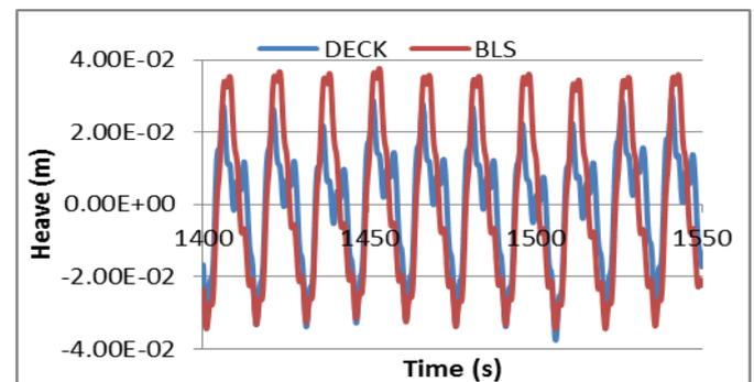
**Fig-5:** Heave response of triceratops without TMD ( $H_{max}=19.2\text{m}$ ,  $T=15\text{s}$ )
