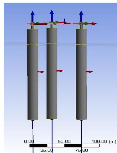
Fig-2: Triceratops modelled in ANSYS AQWA
