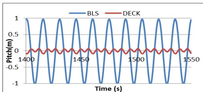
**Fig-3:** Pitch response of triceratops without TMD ( $H_{max}=19.2\text{m}$ ,  $T=15\text{s}$ )
