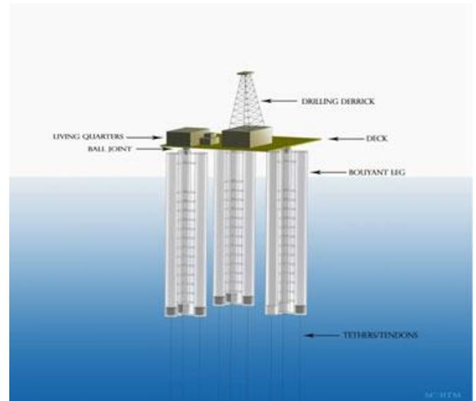
**Fig -1:** Conceptual view of an offshore triceratops
