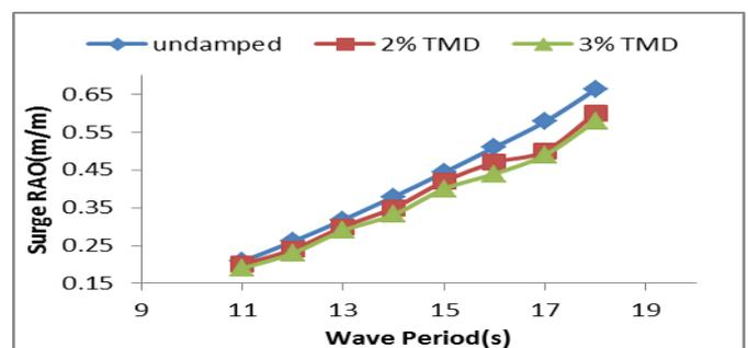
**Fig-6:** Comparison of surge RAO for the BLS unit with and without damper,  $H=19.2\text{m}$
