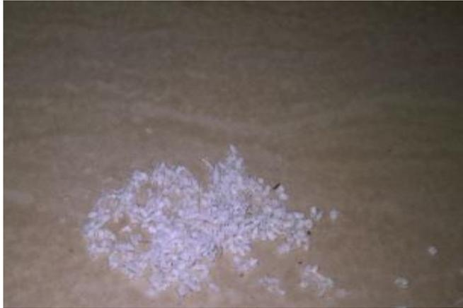
**Fig .2. DISCONTINUOUS BRITTLE CHIPS**
