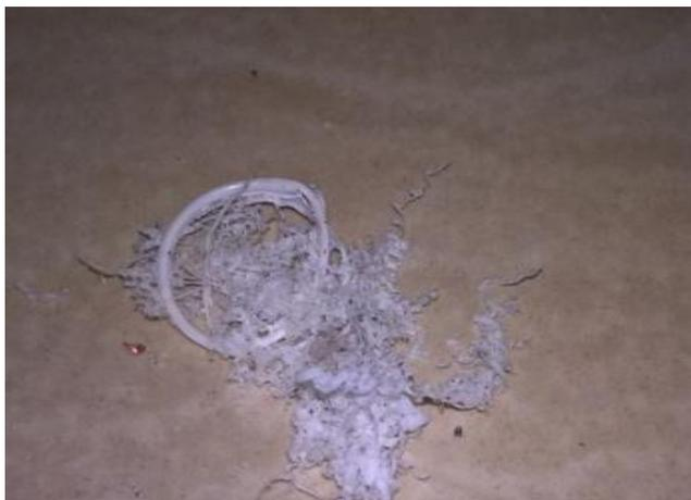
**Fig 4. CONTINUOUS CHIPS**
