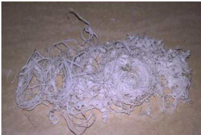
**Fig 3. CONTINUOUS CHIPS**
