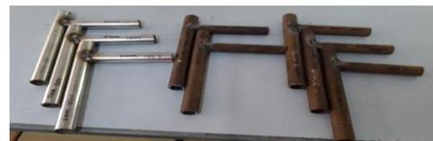
**Fig.5:** Specimen for Bending Test.
