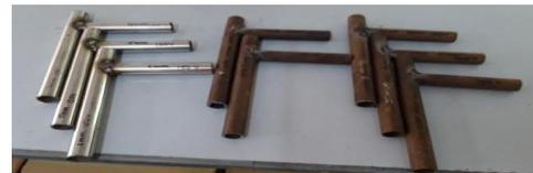
**Fig.5:** Specimen for Bending Test.
