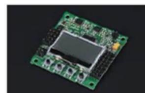
Fig.9. Flight Controller circuit used in quad copter
