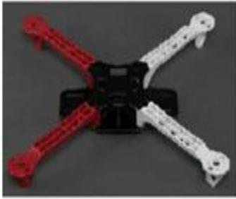
Fig.3. frame of quad copter
