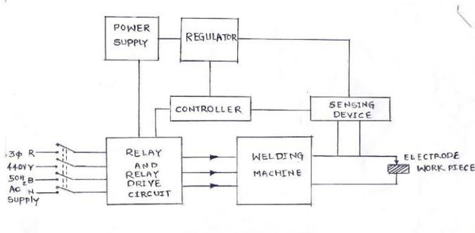
Fig.1. Block Diagram of ESD for Welding Machine
