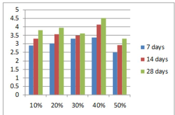
Fig -6: Split tensile strength comparison of GGBS, SS and JY Added concrete.
