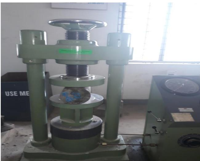
Fig -6: split tensile strength test set-up
