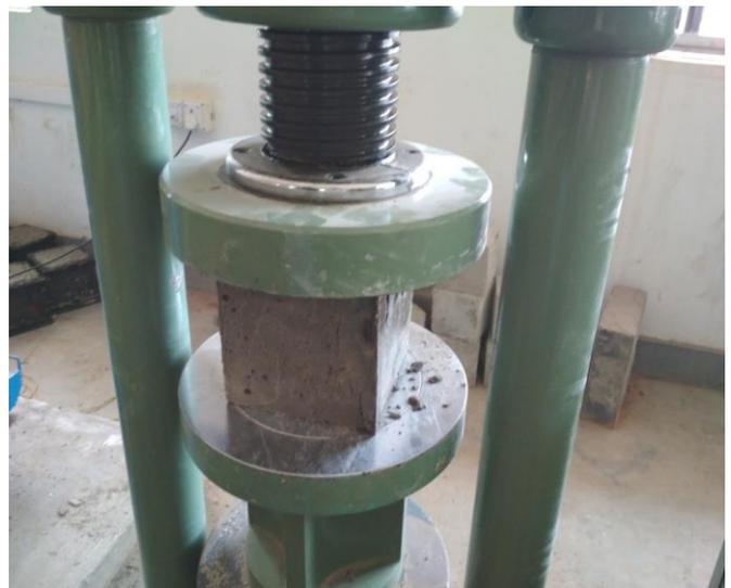
**Fig -4:** Compressive strength test set-up
