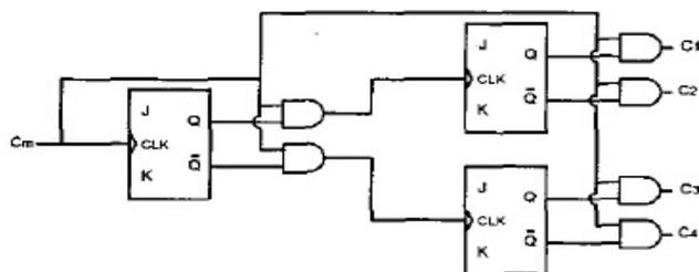
Fig -3: Pulse generation circuit for four interleaved phases
