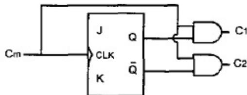
Fig -2: Pulse generation circuit for two interleaved phases
