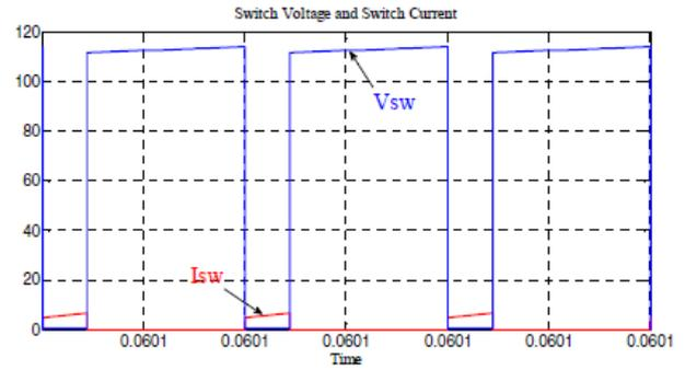
Fig -15: Voltage and current waveform of switches
