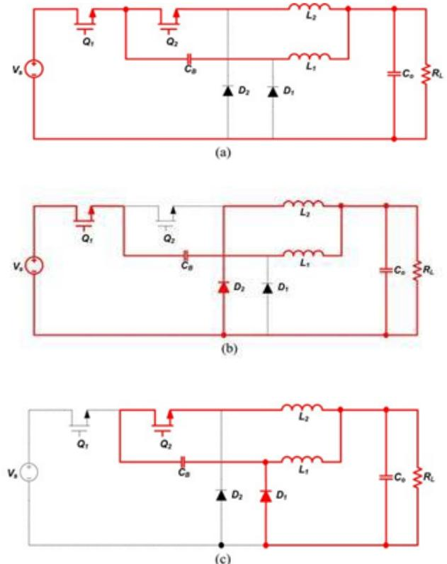
Fig -6: Operation of Circuits when D greater than 0.5.
