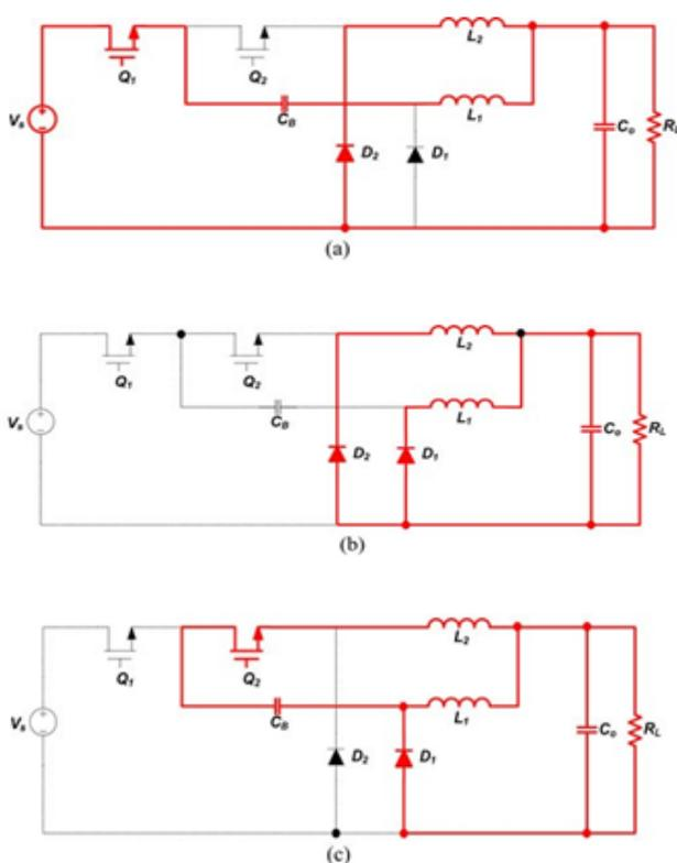
Fig -5: Operating Circuits when duty cycle is less than 0.5
