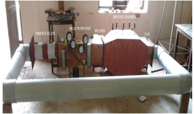
Fig. 4 (a) Experimental setup in horizontal flow arrangement
