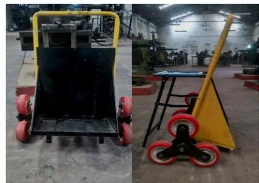
Fig.4.5.2: Final Assembly of easy handling trolley
