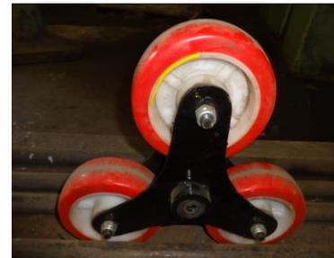
Fig.4.1.1: Assembly of tri-star wheel
