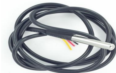
Fig-5: Temperature Sensor (DS18B20)
