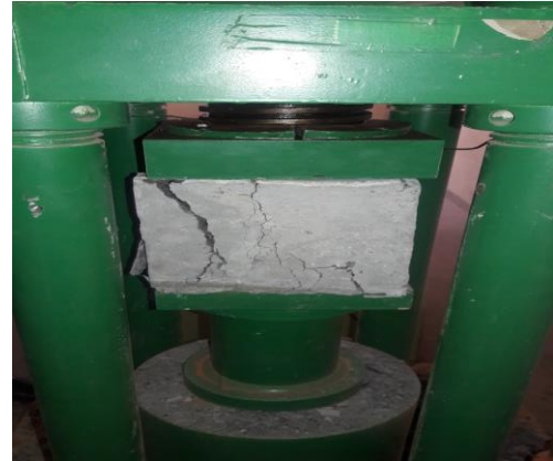
Picture 3: Cracks in Concrete Cube
