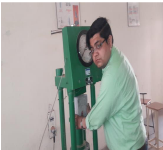
Picture 2: Testing of Concrete Cube Samples
