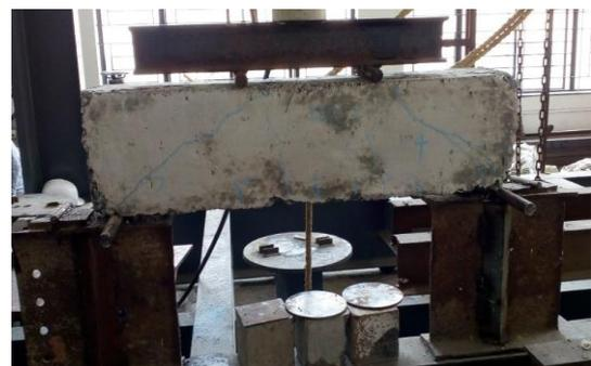
Figure No. 4 Crack Pattern of Beam.
