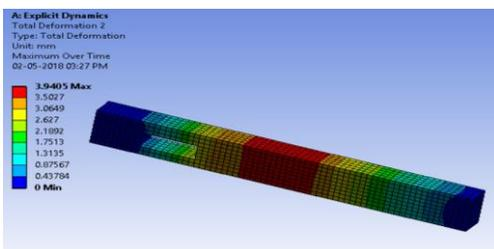
Fig. 3.2 Total deformation non-strengthened beam
