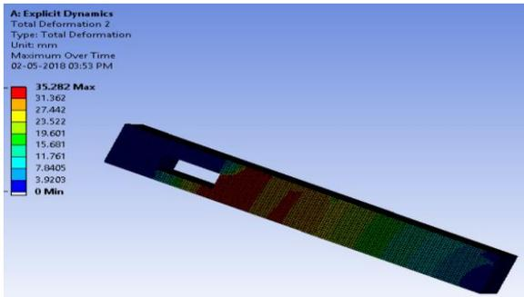
Fig. 3.1 Total deformation non- strengthened beam
