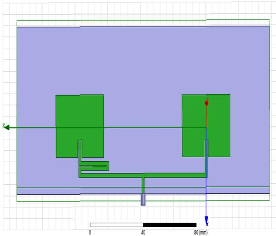
Fig.2. microstrip patch array antenna with transmission line phase shifter of  $-20^\circ$
