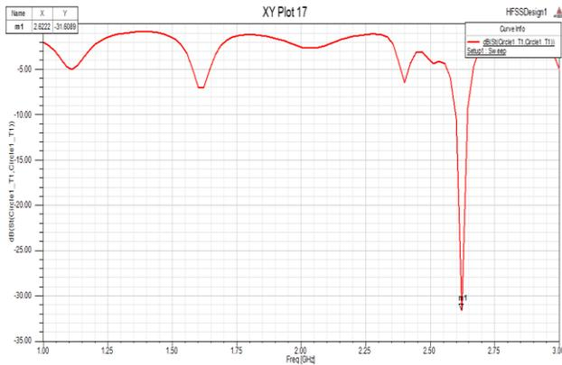
Fig.5. Return loss plot for phase shifter of  $-20^\circ$
