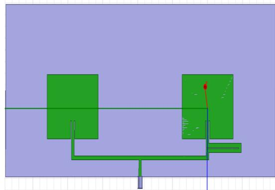
Fig 1.microstrip patch array antenna with transmission line phase shifter of +20°
