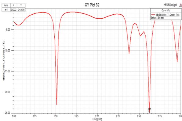
Fig.3. Return loss plot for phase shifter of  $+20^\circ$
