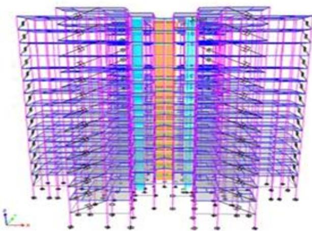
**Figure 3.** 3D view of structure with brace type damper mechanism (Configuration- A)
