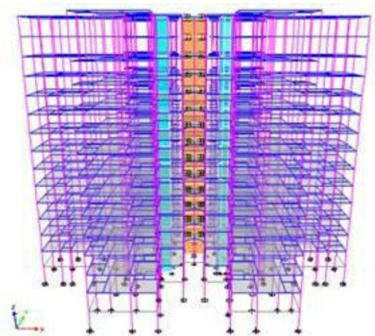
**Figure 4.** 3D view of structure with hybrid coupling mechanism (Configuration- B)
