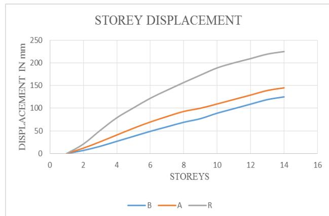
**Chart 3.** Storey displacement for earthquake
