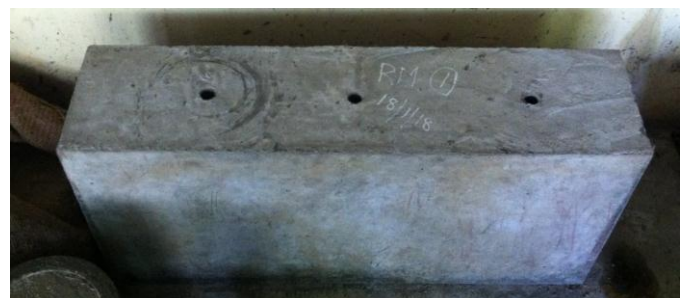
Fig -4: Deep beam casted with hole
