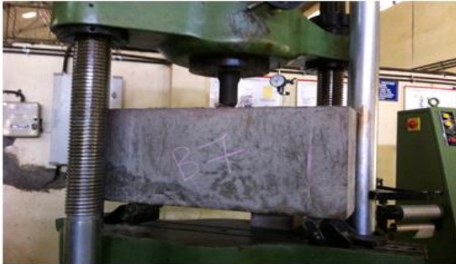
Fig-6: Three point loading arrangement in UTM
