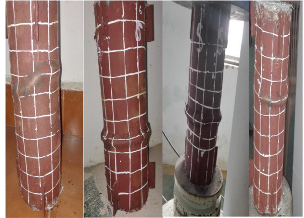
Fig -5: Failure modes of CFSTB circular specimen with diameter 90 mm
