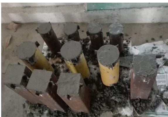
Fig-2 : Casting of CFST specimens
