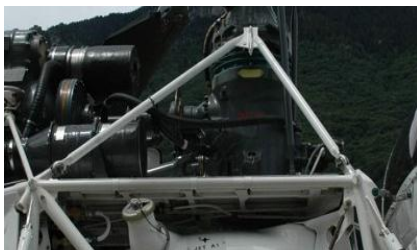
Fig -1: A-Frame as assembled on the helicopter
