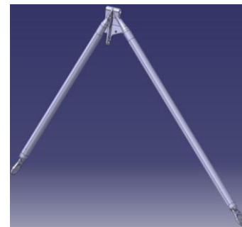
Fig -3: A-Frame assembly
