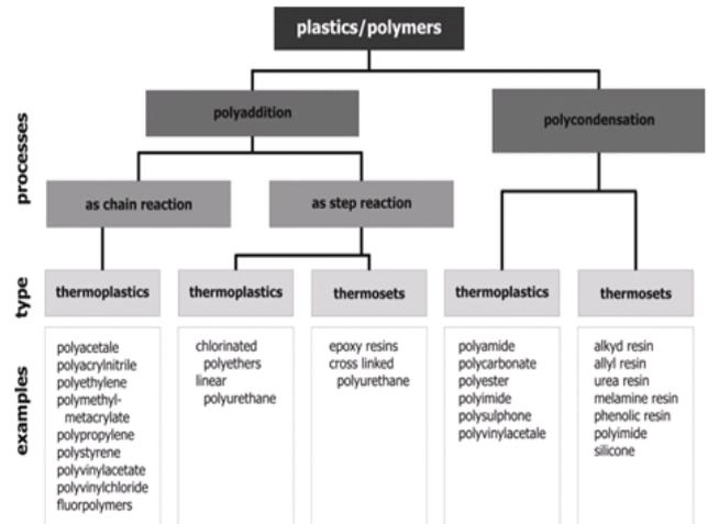
Figure 1: Process for generating Plastics and Examples [2011 Wiley-VCH Velar et al.]
