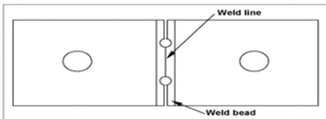
Figure 4: Tensile welded joints( BS EN 12814-2)
