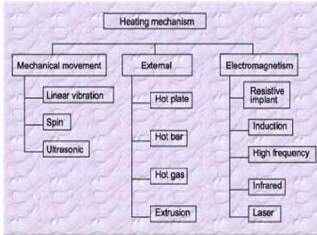
Figure 2: Welding processes for thermoplastics.
