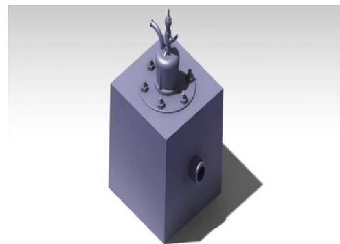
Fig -6 Air box for supply biogas to engine
