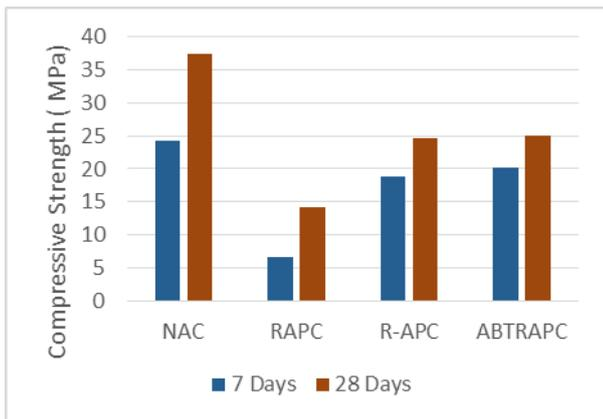
Fig.1. Compressive strength for all mixes
