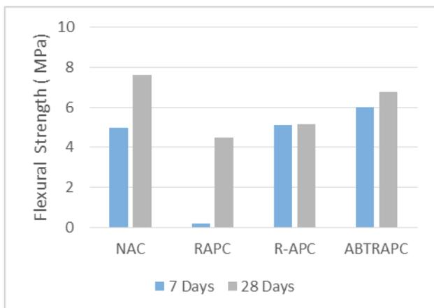
Fig.2. Flexural strength for all mixes
