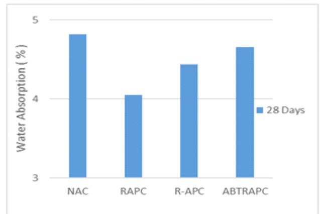
Fig.4.Water absorption test for all mix
