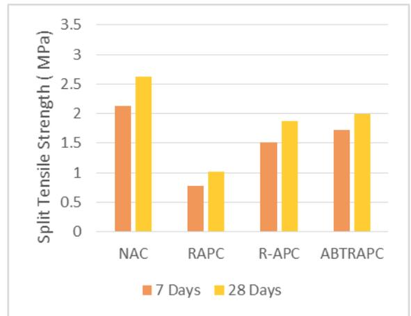
Fig.3.Tensile strength for all mixes
