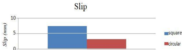
Chart -2: Slip of square and circular CFST column specimens
