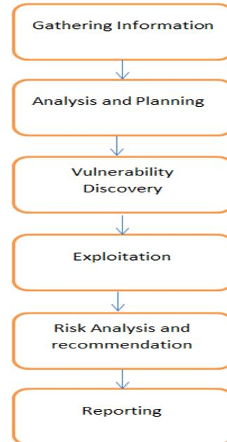
**Fig-1:** Penetration testing phases
