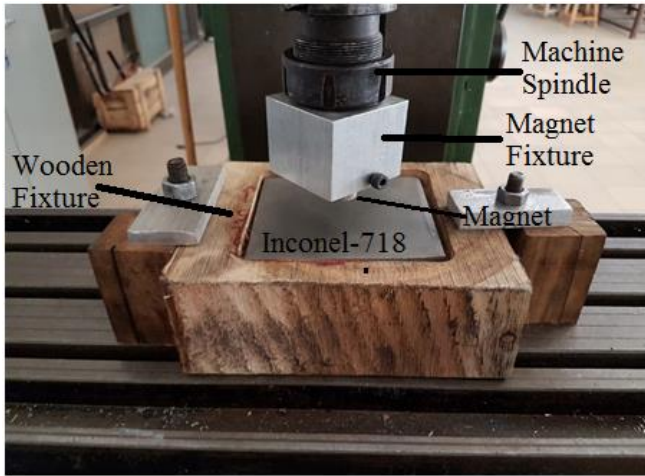
Fig -1: Photograph of Experimental Set up and wooden fixture.
