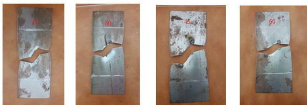
Fig - 7: 45° and 60° inclined crack with and without weld after testing
