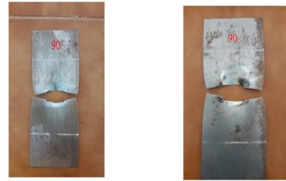
Fig - 8: 90° inclined crack with and without weld after testing
