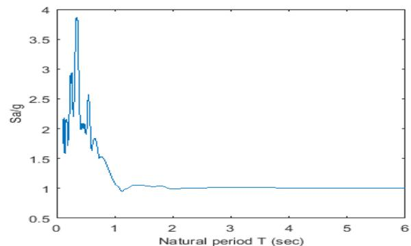
Figure 12: India-Burma (1995) Acceleration Response Spectra at Diphu Station
