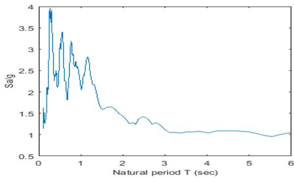
Figure 5: Bhuj (2001) Acceleration Response Spectra at Ahmedabad Station
