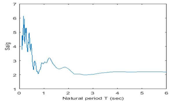
Figure 10: India-Burma (1988) Acceleration Response Spectra at Bokajan Station
