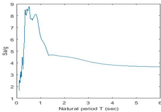
Figure 7: Chamoli (1999) Acceleration Response Spectra at Gopeshwar Station
