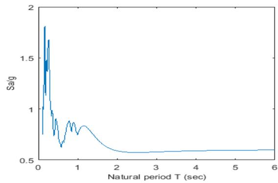
Figure 9: India-Burma (1987) Acceleration Response Spectra at Laisong Station
