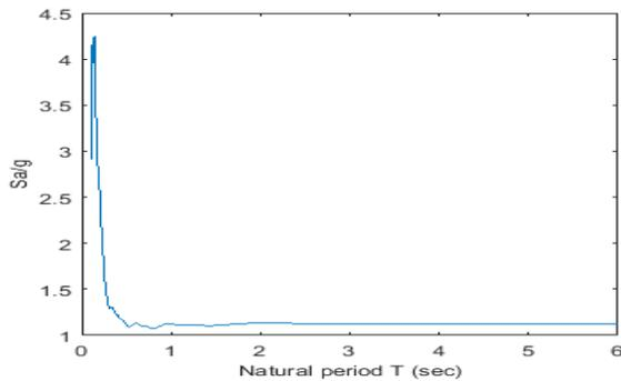
**Figure 14:** NE-India (1986) Acceleration Response Spectra at Ummulung Station
