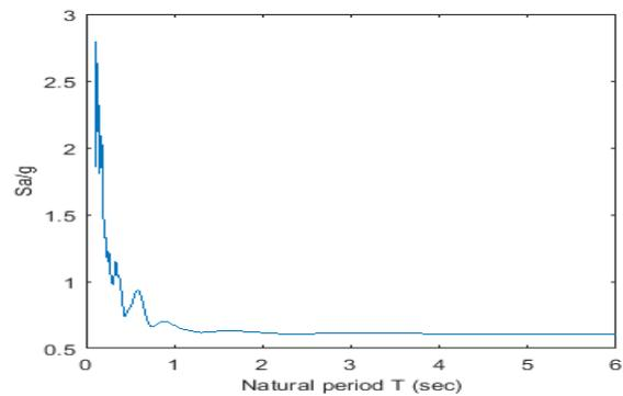
Figure 11: India-Burma (1990) Acceleration Response Spectra at Laisong Station
