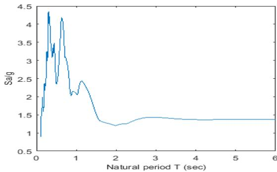
**Figure 13:** India-Burma (1997) Acceleration Response Spectra at Jellalpur Station
