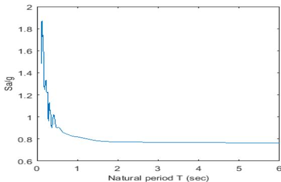
**Figure 15:** Xizang India (1996) Acceleration Response Spectra at Ukhimath Station
