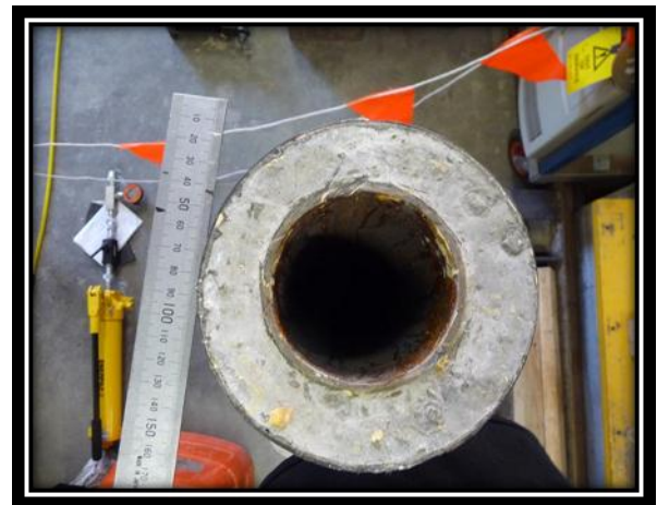
Fig -1: Concrete filled double skin steel tube [4]
