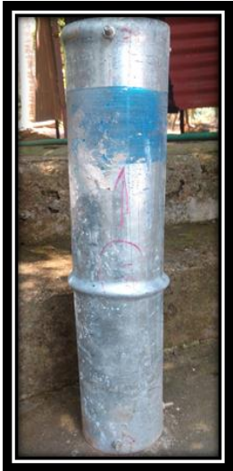
(a) Local buckling was observed at the top portion and also 36cm from the top.
