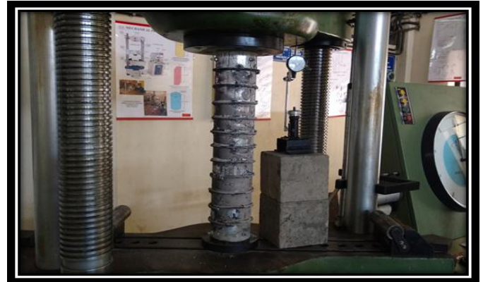
Fig -4: Experimental test setup of column specimens
